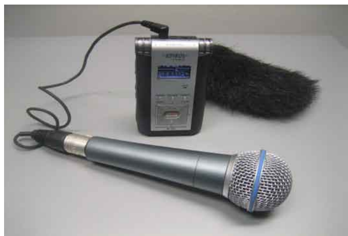
Figure 3. R09 with external Shure Beta 58A dynamic microphone
